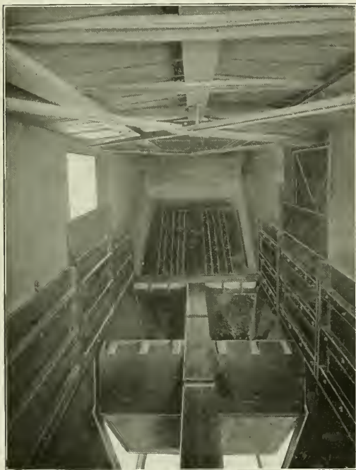
Interior of the Grand Trunk Hopper Bottom Box Car.
